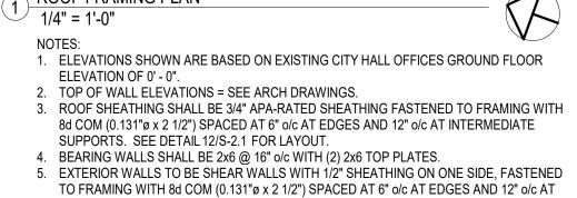
INTERMEDIATE SUPPORTS WITH (2) 2x6 TIÉ DOWN STUDS AT ENDS. BOTTOM PLATE ATTACHMENT TO BE (2) 16d COM (0.162"ø x 3 1/2") AT 16" o/c OR 1/2"ø SILL ANCHORS AT 48"o/c TO FOUNDATION. SEE SHEAR WALL DETAIL 13/S-2.1. 6. "#J + #K" INDICATE NUMBER OF 2x6 JACK AND KING STUDS, RESPECTIVELY, REQUIRED.
